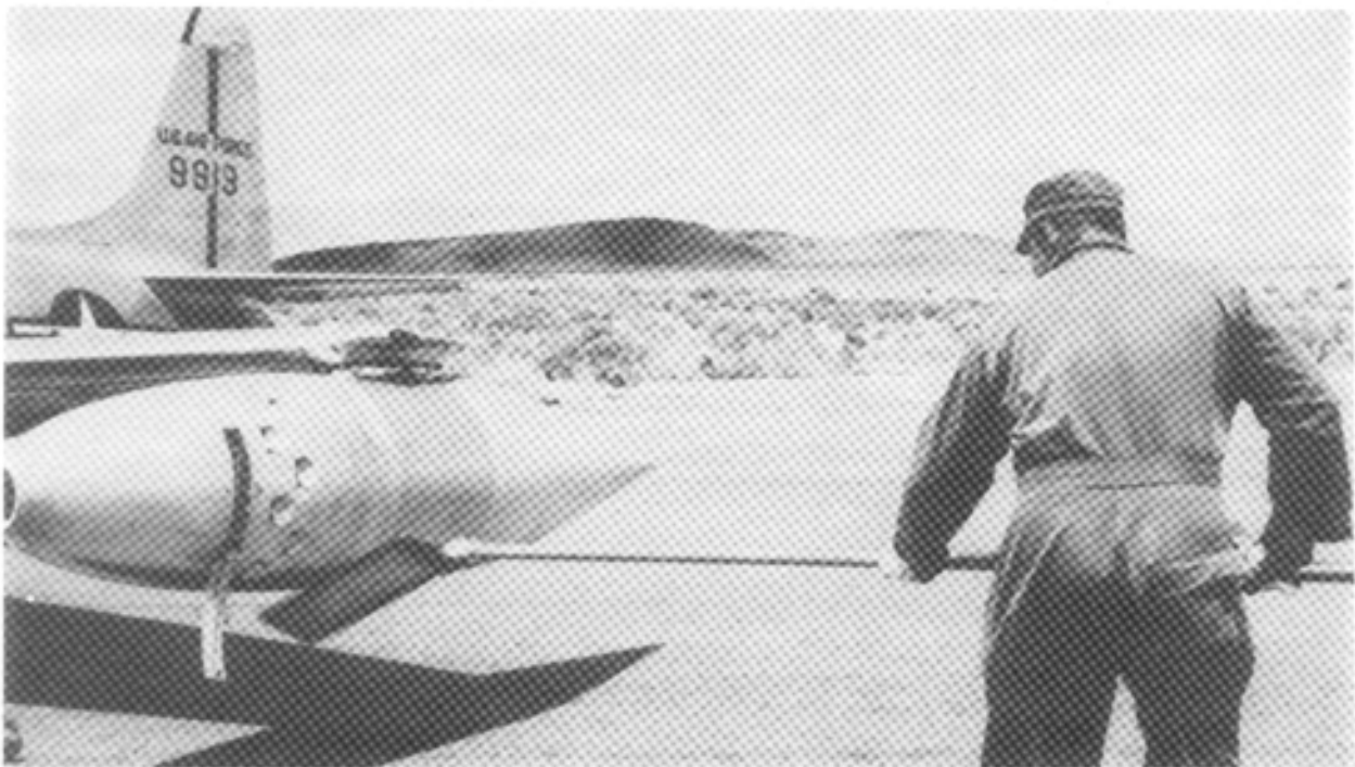
Figure 5-6: MEMBER OF THE SAMPLE REMOVAL TEAM REHEARSES TECHNIQUE USED IN REMOVING WING-TIP CLOUD SAMPLES
