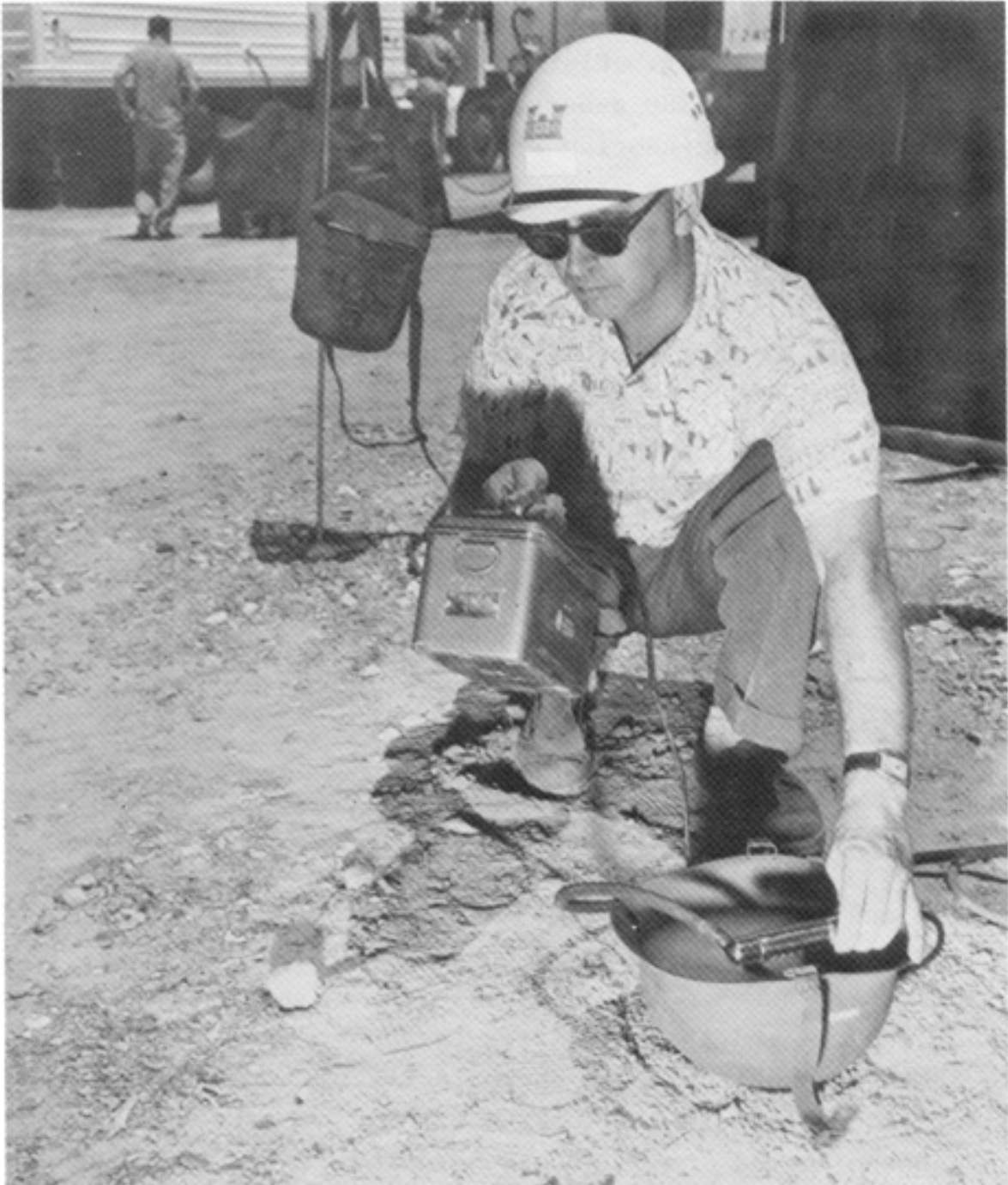
Figure 2-3: PARTICIPANT FROM ENGINEER RESEARCH AND DEVELOPMENT LABORATORIES DETERMINES THE RADIATION CONTENT OF CONTAMINATED WATER DURING PROJECT 50.4, EVALUATION OF WATER DECONTAMINATION METHODS
