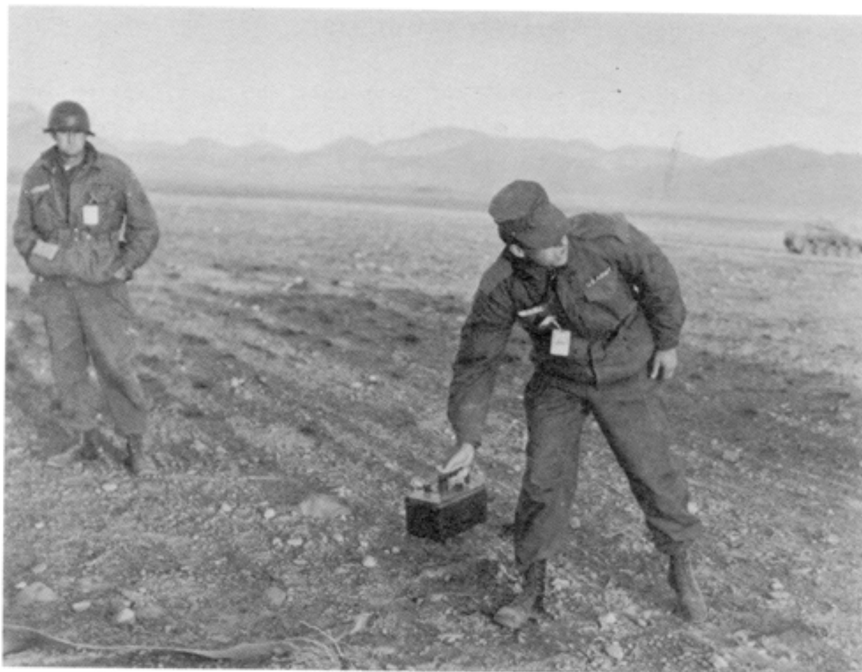
Figure 3-3: RADIOLOGICAL SAFETY PERSONNEL OF THE 50TH CHEMICAL SERVICE PLATOON MEASURES THE RADIOACTIVITY OF A PIECE OF METAL FROM THE APPLE 1 TOWER
