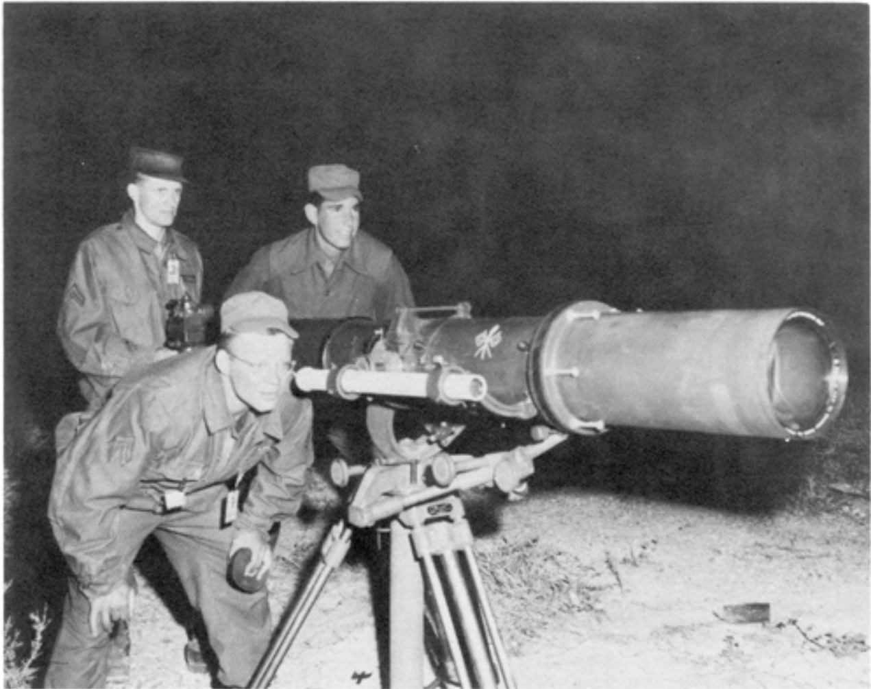
Figure 3-2: SIGNAL CORPS TROOPS POSITIONING LONG-RANGE TELEPHOTO LENS TO PHOTOGRAPH MOTH DETONATION FROM NEWS NOB
