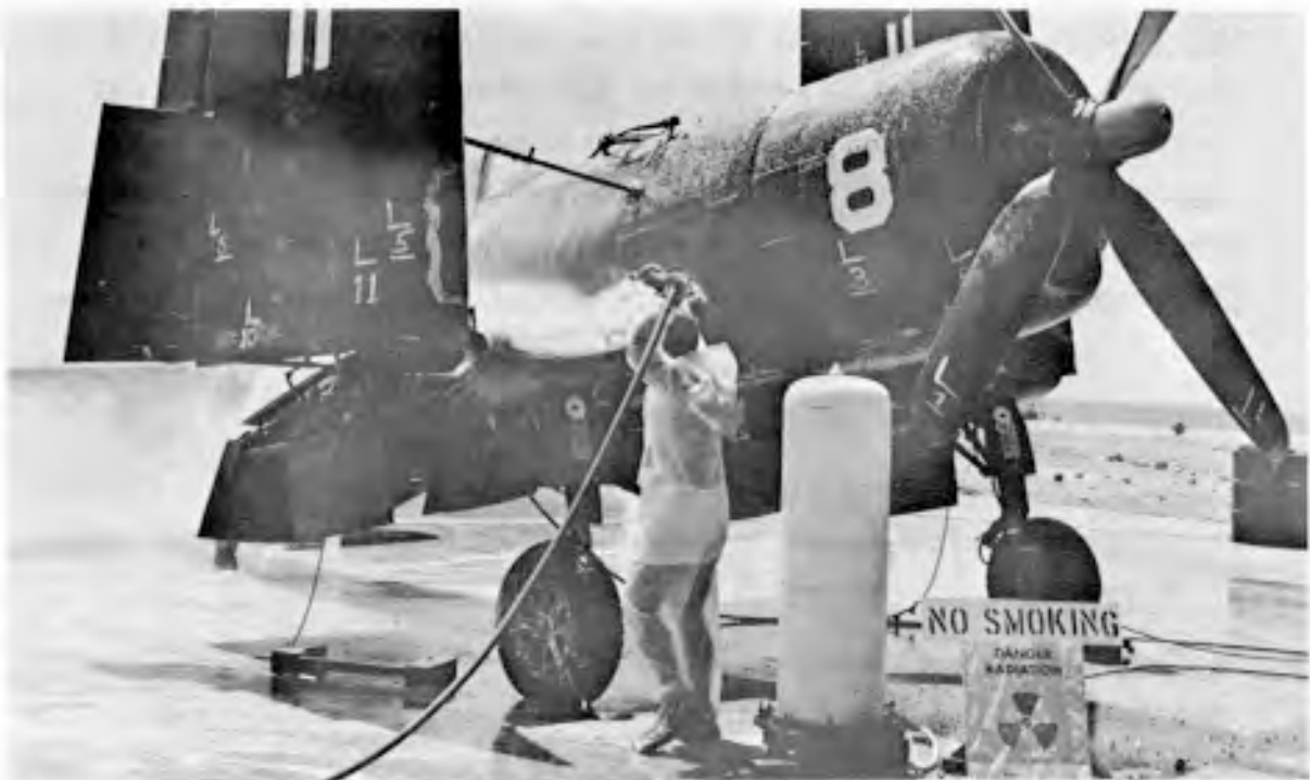
Figure 51. Project 6.4 test aircraft being decontaminated, CASTLE.
