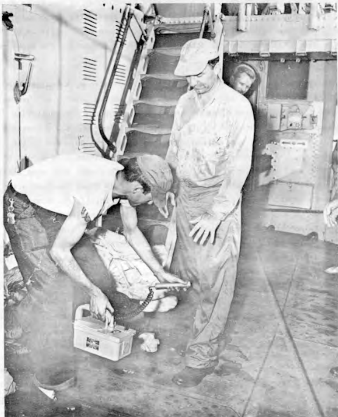
Figure 35. Personnel monitoring after removal of contaminated clothing (also note removable covering on deck and ladder in background), CASTLE.
