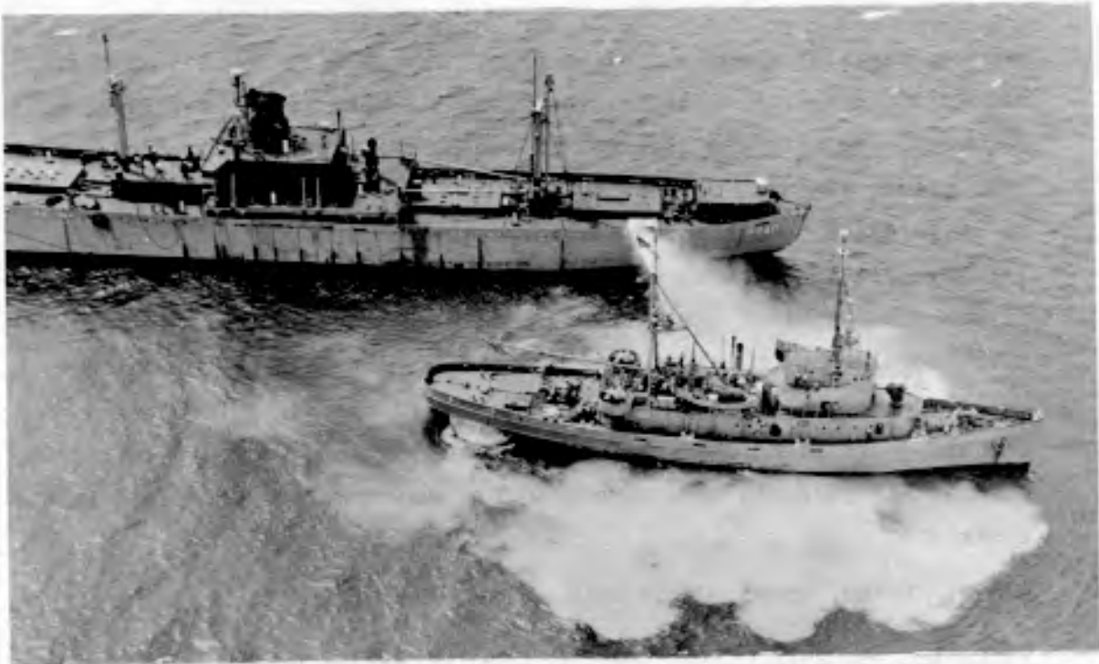
Figure 48. Decontamination hosedown of YAG-40 ( USS Granville S. Hall ) by the USS Molala (ATF-106), CASTLE.
