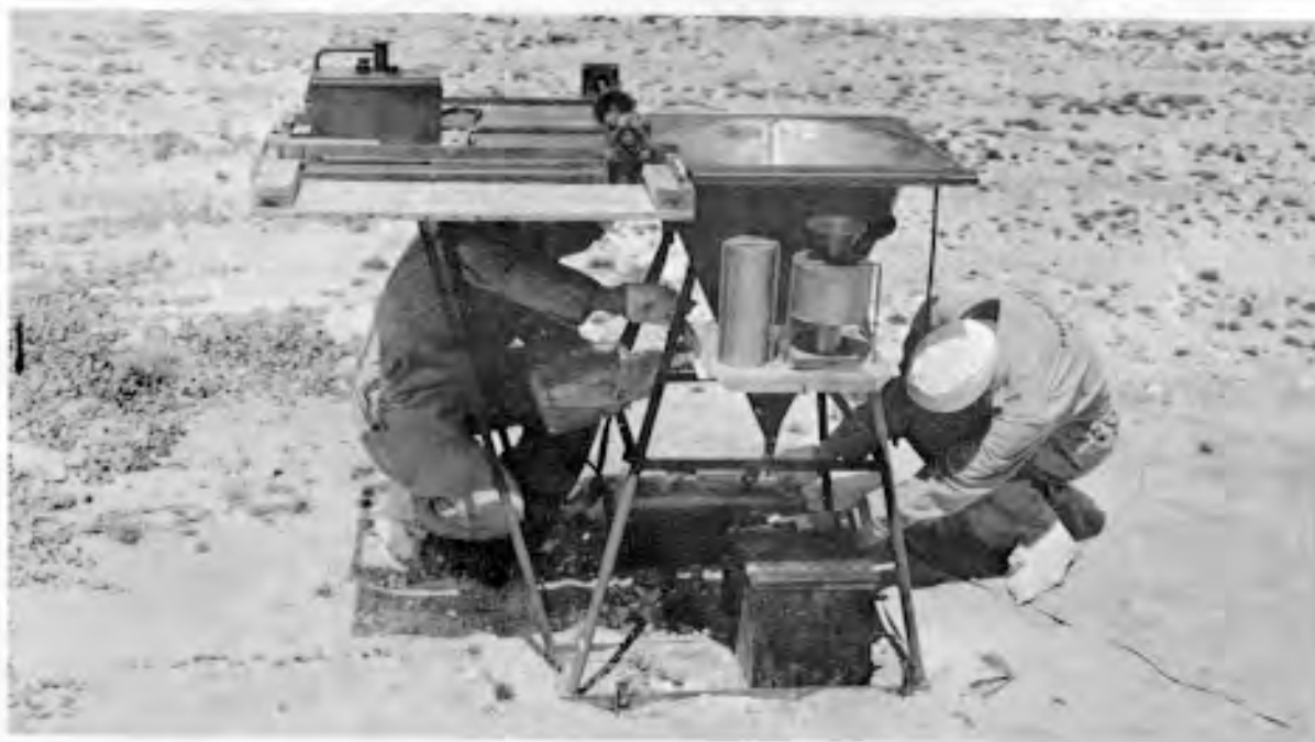
Figure 46. Preparation of fallout collector tray, CASTLE.
