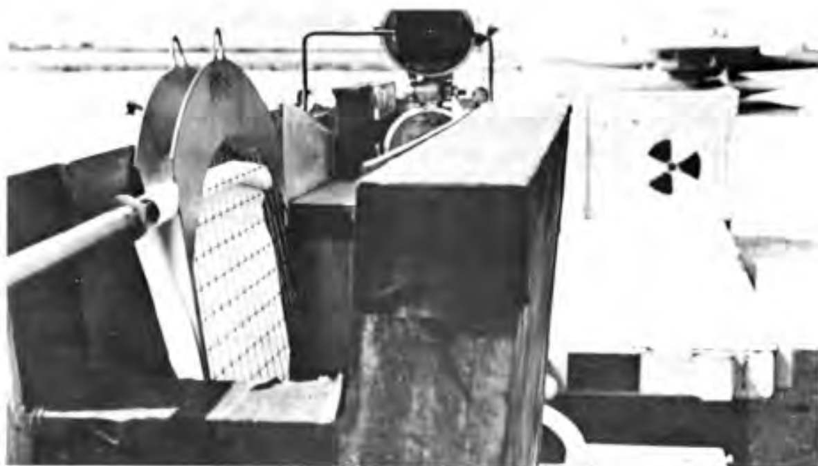
Figure 31. Filter paper being rolled, CASTLE.
