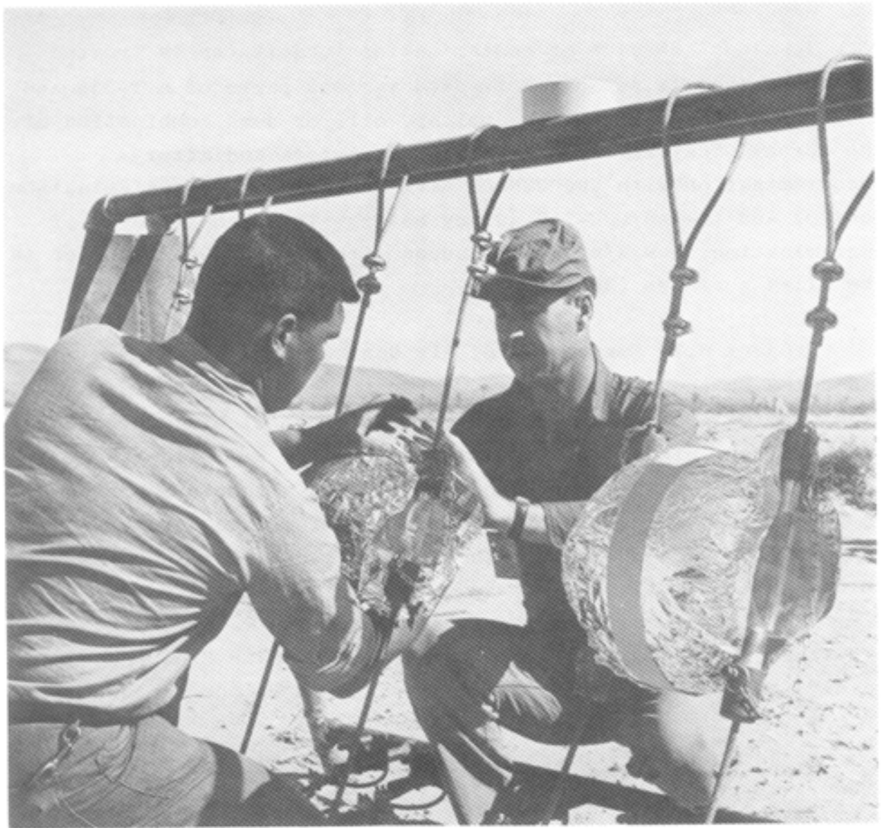
Figure 5-3: PROJECT 4.4 PERSONNEL PREPARE LUCITE SPHERES USED TO MEASURE GAMMA RAY DEPTH DOSE
