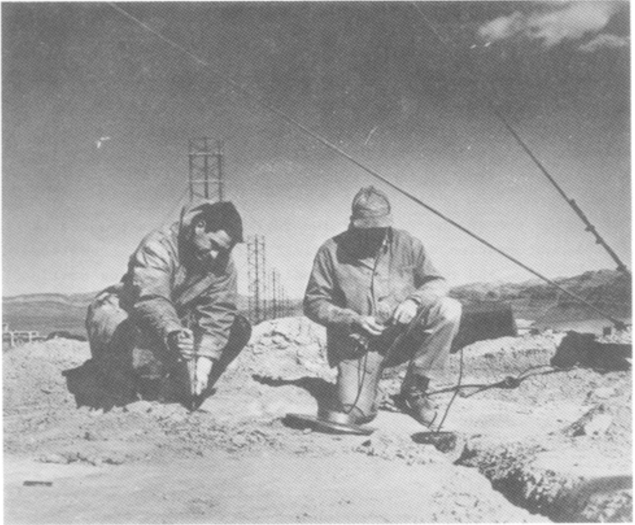
Figure 2-1: PROJECT 1.7 PERSONNEL INSTALL ACCELEROMETERS ALONG THE BLAST LINE
